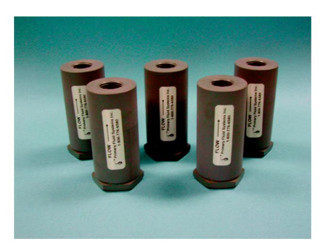
ACCU-VENT automatic degassing valves are designed to automatically vent gases and vapors that are commonly released from chemicals such as Sodium Hypochlorite, Sulfuric Acid or Hydrogen Peroxide.
