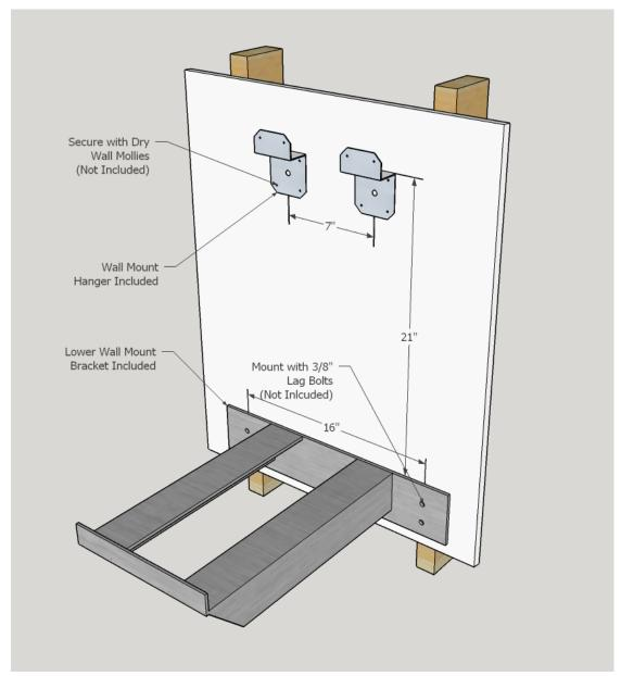
**5.1 POLY CONTAINMENT/MOUNT SHELF** Once brackets are secured to wall as shown above. Place the polyethylene containment shelf through the handhole molded in the upper back. The lower basket should fit snugly into the low bracket assembly.
